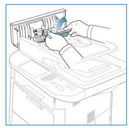
4. If necessary, use two hands to raise the duplex cover and pull any jammed originals gently out of the *document feeder*. If you see no paper in this area, go to the next step.
